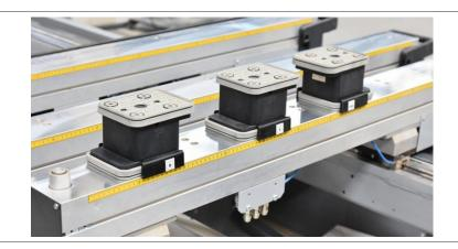
These hold your workpiece in place during cutting. Inspect for cracks or loss of suction power and replace worn pods to ensure stability during operations.
