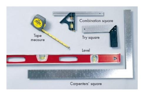
Fig. 198: Measuring and marking tools
