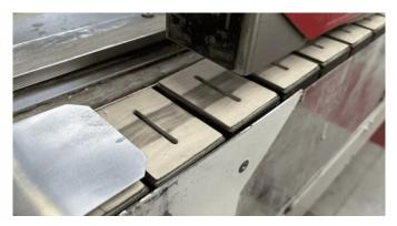
Fig. 342: Checking the Conveyor Belt for Wear
