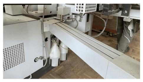
Fig. 339: Lubricating Moving Parts
