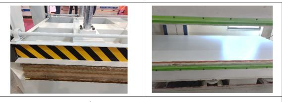
Panel inside a cold/hot press machine with even pressure distribution
