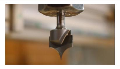
Router bits are the cutting tools that shape your materials. Regularly inspect for wear and replace them promptly to maintain cutting precision. Store them in a dry, organized space to avoid corrosion.
