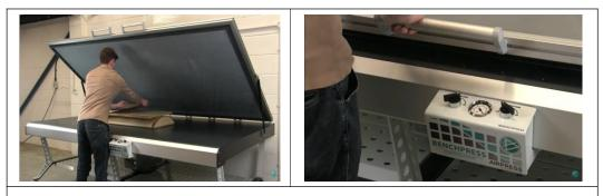
Small wooden pieces being positioned for veneer application in a vacuum press
