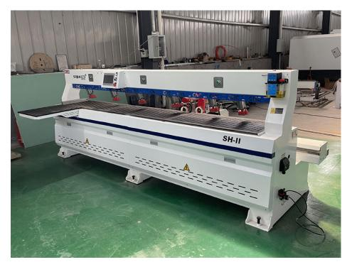
Fig. 348: CNC Side Holes Drilling Machine
