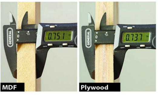
Fig. 299: Measure dimensions of material
