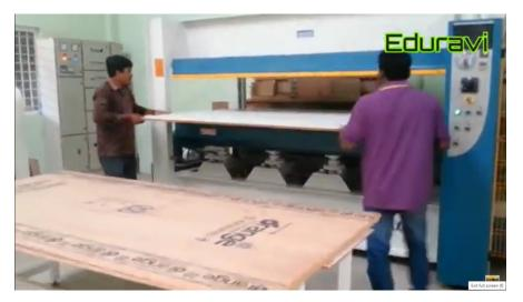
Fig. 179: A worker checking adhesive spread and pressing uniformity on a test panel
