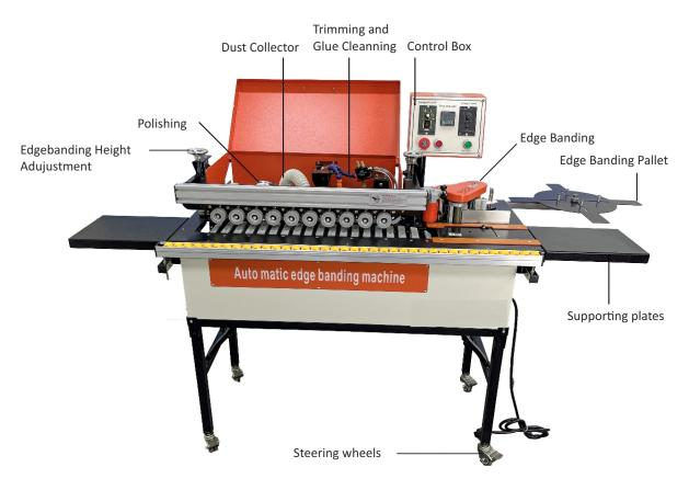
Fig. 176: Edge Banding Machine Setup and Calibration
