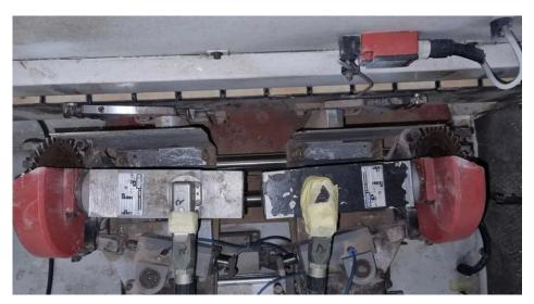
Fig. 340: Inspecting Trimming Blades and Cutters
