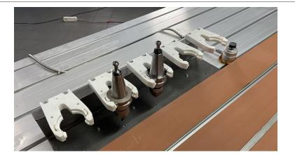
For routers with automatic tool changers, tool forks must be aligned and free from cracks. Regular alignment checks and timely replacements are essential for seamless operations.
