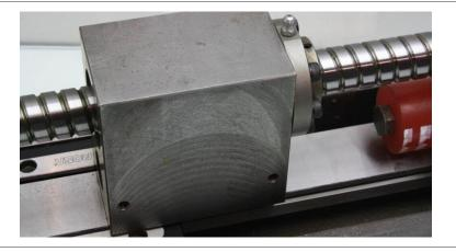
These components ensure precise motion. Clean guide rails and screws to prevent debris buildup and apply the recommended lubricant sparingly but consistently.
