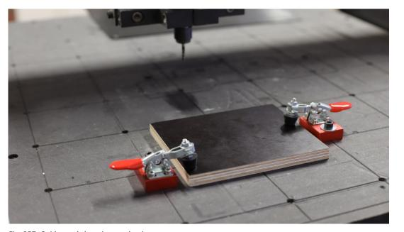
Fig. 357: Guides and clamping mechanisms
