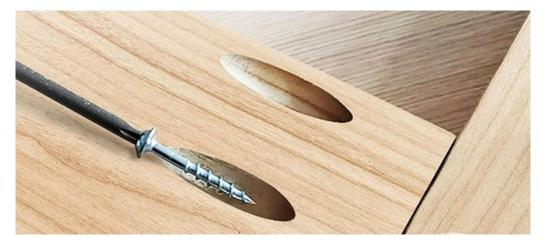
Fig. 345: Pocket hole drilling
