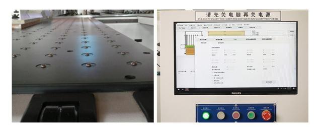
Fig. 173: CNC beam saw machine
