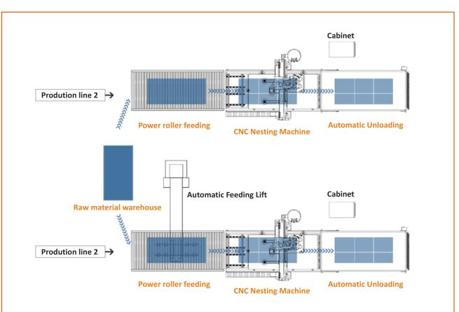
Fig. 88: CNC Nesting Machine with Drilling Machine
