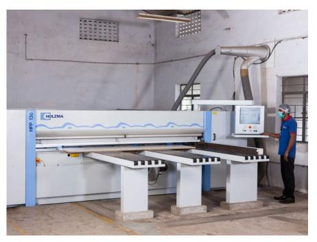
Fig. 110: Beam Saw for production
