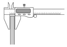
Fig. 278: Calliper measuring thickness
