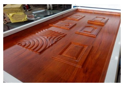
Fig. 283: Inspecting a laminated MDF panel after vacuum pressing
