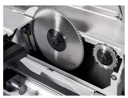
Fig. 318: Sliding table panel saw
