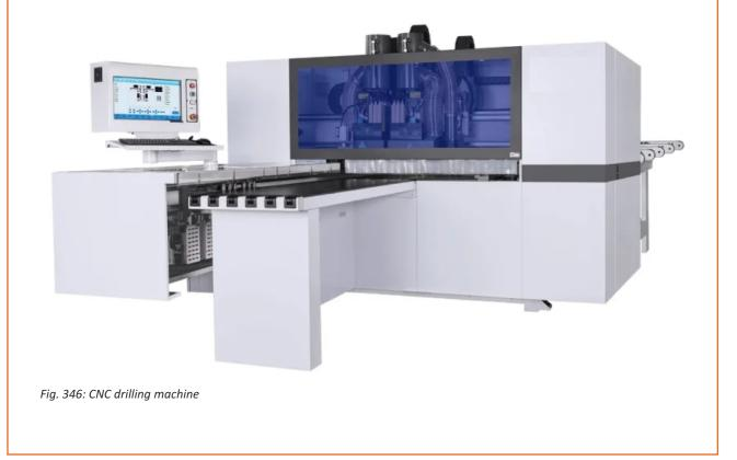
CNC drilling center with three drilling groups (2 from above and 1 from below) for drilling from 6 sides and a grooving saw is designed for high-precision drilling of through and blind holes in the ends and planes of furniture panels, which allows processing any additive maps in one pass of the part. The machine is equipped with two milling units for milling both simple straight grooves, such as a groove for the back wall or the bottom of a box, and profiling.
