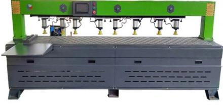
Fig. 344: CNC Drilling Machine Operations in Panel Works furniture
