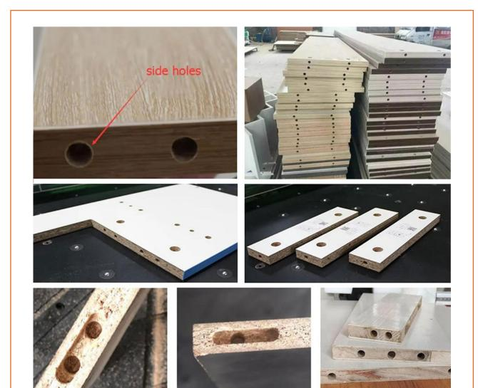
Fig. 352: Side holes in workpieces
