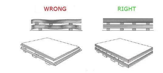
*Fig. 298: Correct way of stacking/storing the material*
