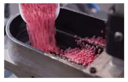
Fig. 207: Cleaning of PUR Edgebanders
