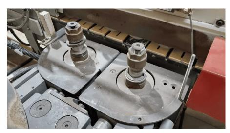
*Fig. 338: Checking the Alignment of the Pre-Milling Unit*
