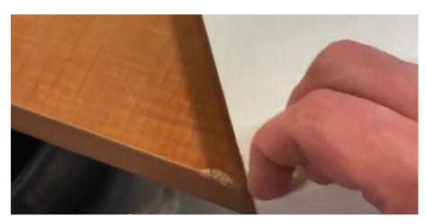
Fig. 181: A worker checking the edge band adhesion and trimming accuracy on a test panel
