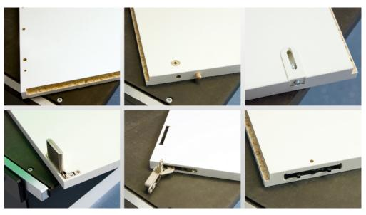
Fig. 189: Making precise holes in panels for hinges, dowels, and fittings
