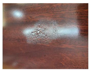
Fig. 277: Identify defects like bubbles, wrinkles, or uneven surfaces
