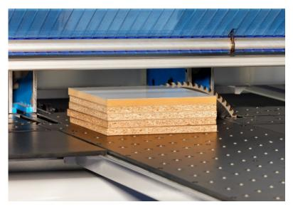
Fig. 295: Using a beam saw machine
