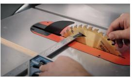
Fig. 114: Checking table saw blade alignment
