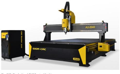
Fig. 360: Single-Head CNC Router Machine
