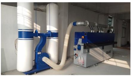
Fig. 105: Wood dust collector
