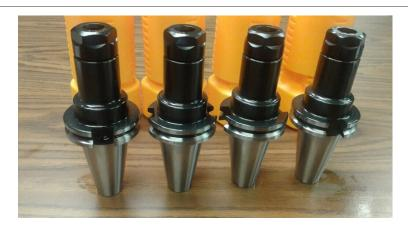
Critical for holding bits securely, collets and tool holders must be cleaned and checked for deformation regularly. Damaged holders can lead to operational inefficiencies and safety risks.
