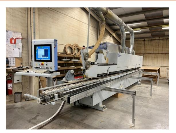
Fig. 323: Effective collaboration with the machine operator for edge banding process
