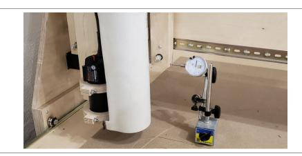
Calibration and Alignment: Maintain precision by recalibrating axes and aligning tools to specifications.
