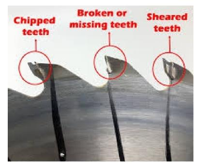
Fig. 223: Types of tooth damage
