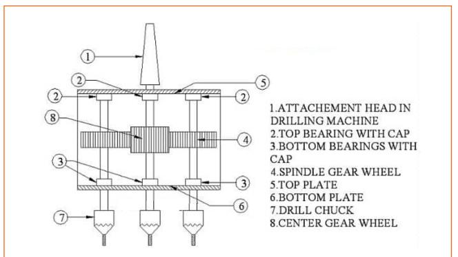
Fig. 350: Multi-spindle drill head
