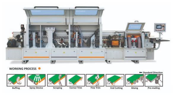
Fig. 122: Machine specification
