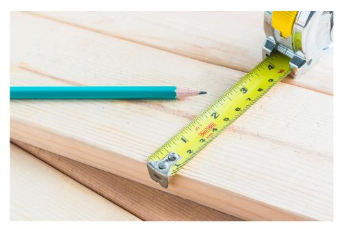
*Fig. 197: Accurate Measurement and Marking of wooden panel*
