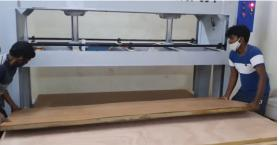
Fig. 279: Aligning veneer sheets on a wooden board
