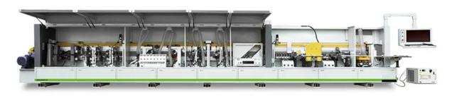
Fig. 334: Laser edge banding machine
