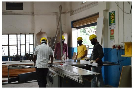
Fig. 158: Using PPE during machining operation
