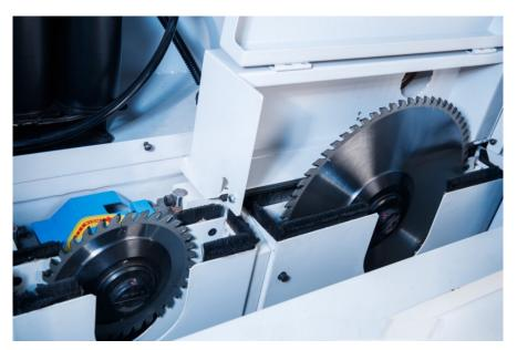
Fig. 146: CNC panel saw
