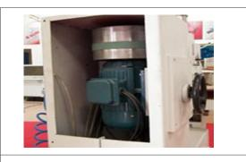
Spindle drive assembly easily accessible for belt tension & maintenance.
