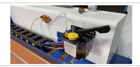
Lubrication: Friction is the enemy of precision. Apply manufacturer-recommended lubricants to ball screws and linear guides to ensure seamless motion.
