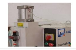
Up & down movement of work table to set work piece thickness.
