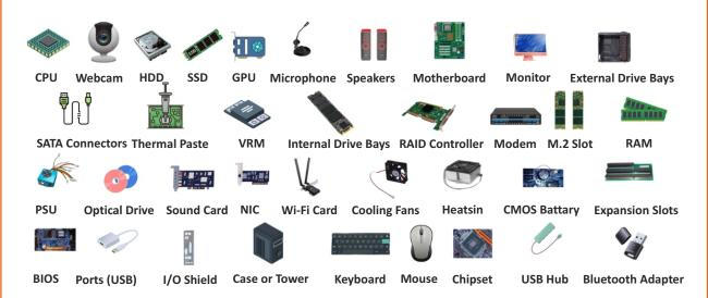
Fig. 77: Parts of a computer
