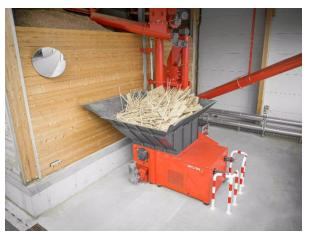
Fig. 233: Chipper and shredder for wood waste
