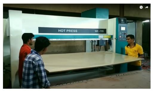
Fig. 284: Inspecting a finished laminate board after unloading
