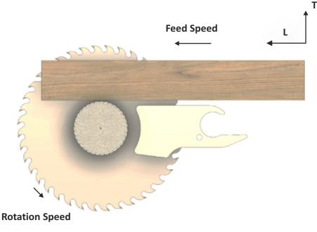
Fig. 84: Adjusting feed rate
