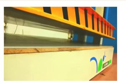
*Fig. 282: Removing a bonded plywood panel from the cold press*
