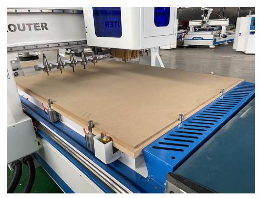
Fig. 296: Using a nesting cutting machine
