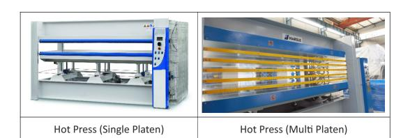
Loading: Ensure the worktable is clean L and free from dust or debris. Align the f panel properly to avoid misplacement and g ensure even pressing. Use lifting aids (e.g., b vacuum lifters, roller conveyors) to h minimize manual strain. Position the l material centrally to distribute pressure lo evenly. Apply protective sheets if required g to prevent surface damage.
