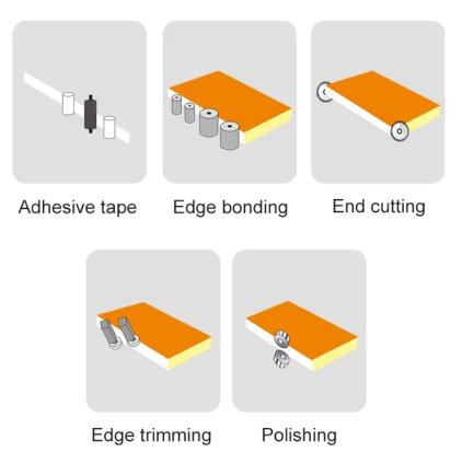
Fig. 177: Automatic banding and trimming machine
